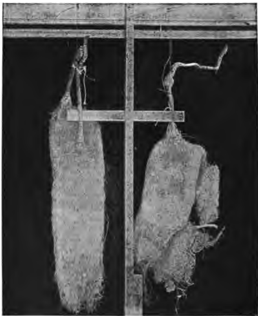
FIG. 45. — Showing the roots of European larch removed from a 6-inch tile drain, which they had effectually clogged.
